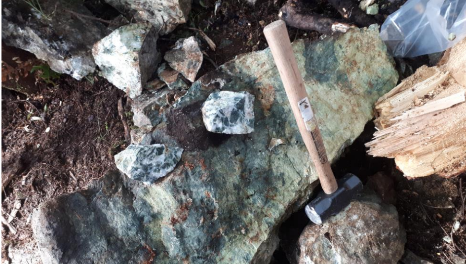
Photo 3. Green malachite staining at sample site 32306, lower Sunset adit. This sample site returned 5100 ppm Cu and 6.04 ppm Ag. Photo taken by the author, November 12, 2018.
