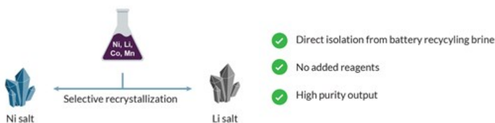
Figure 1. Telescope's recrystallization technique separates high purity materials from battery recycling brines.
