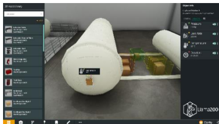
Image of LlamaZOO's Clarity product demonstrating equipment captured from 3D laser scans and represented as a virtual environment with IoT sensor data.
