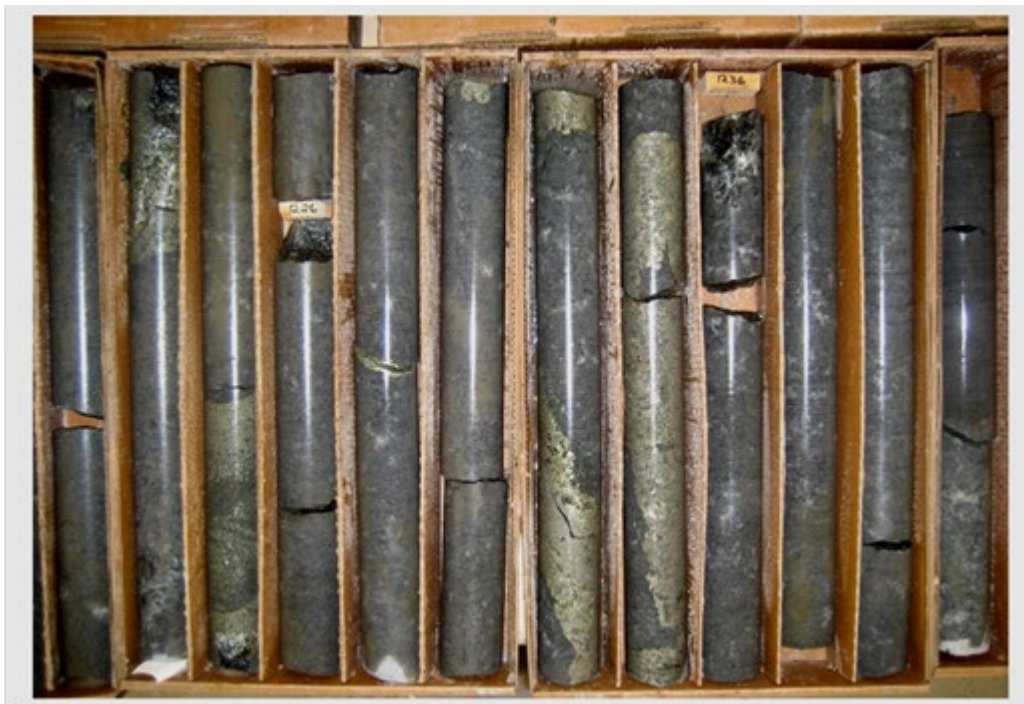
Figure 7. Core photo showing a Cu-Ni mineralized zone in drill hole SK09-2 between 372.4 to 376.1m (3.7m) which grades 2.3% Cu, 0.8% Ni and 1189 ppb PGE. Sulfide mineral assemblages include chalcopyrite, pentlandite and pyrrhotite. Hole drilled by EMI (2009).
