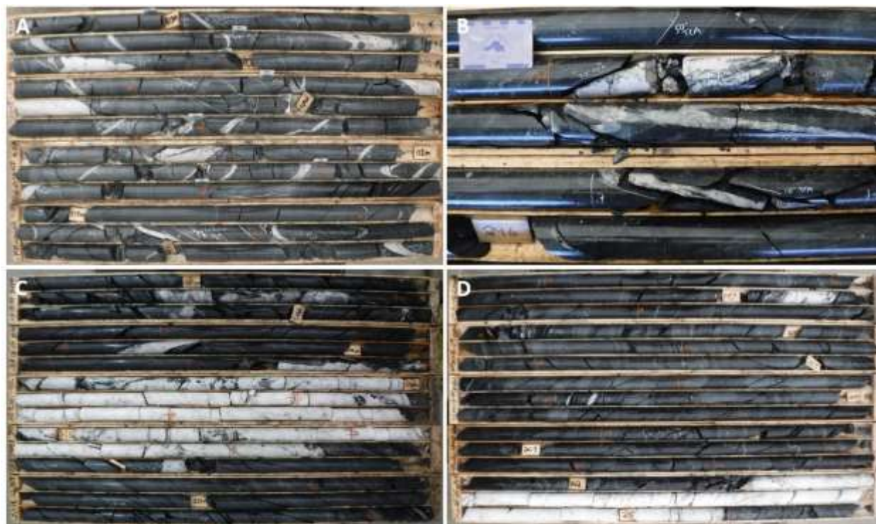
Figure 27: A) MM-18-02 representing a zone of increased quartz veining from 102m to 119m. Veins are dominantly subparallel Low-angle veins and some AC veins. B) MM-18-04 representing two types of quartz veins, laminar vein subparallel to bedding at the top and two Low-angle veins beneath. C) MM-18-04 saddle reef vein from 210.65m to 217.35m. Vein had sharp contacts and local zones of massive arsenopyrite and minor pyrite. D) MM-18-05 following up on the MM-18-04 saddle reef vein intercept. The intersection of the saddle reef vein is from 212.5m to 215.35m
