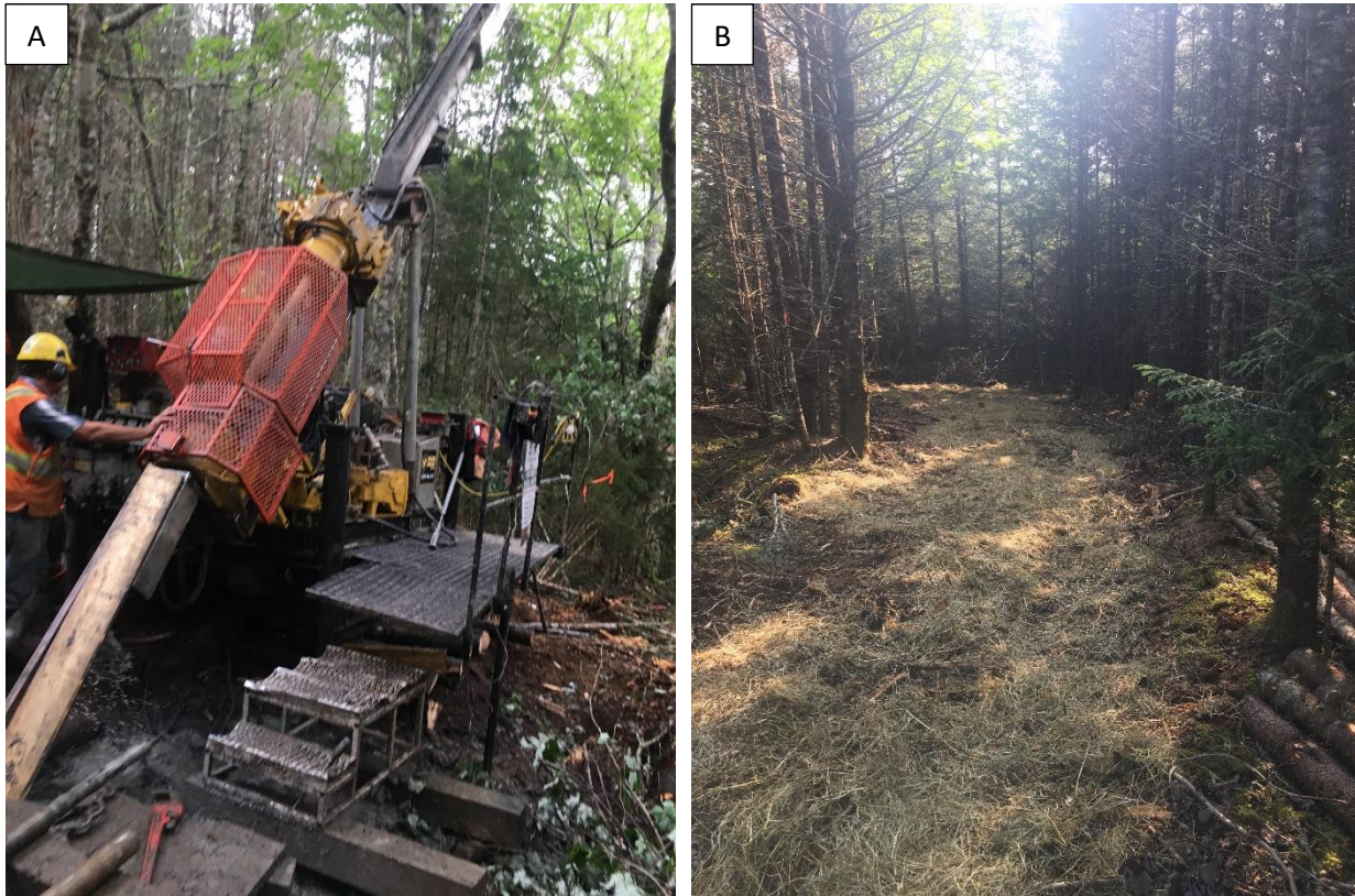
Figure 33 a) Photograph of the drill set up on a Probe Metals drill site b) Photograph of one of the Probe Metals clean drill sites post drilling
