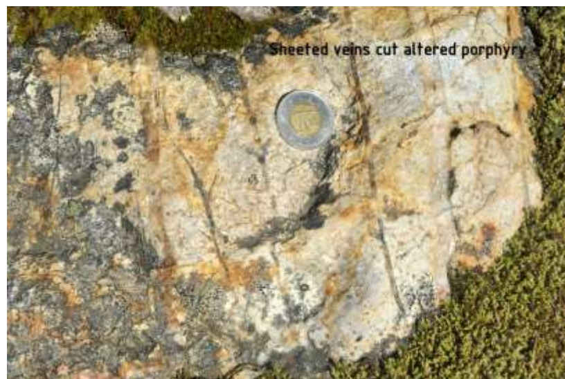
Figure 42. Centimetre scale, parallel (sheeted) late-stage quartz veins filled by translucent to pale grey quartz, sericite and pyrite. These veins are thought to host gold.
