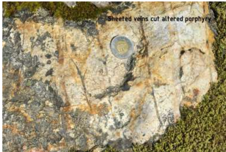
Figure 39. Centimetre scale, parallel (sheeted) late-stage quartz veins filled by translucent to pale grey quartz, sericite and pyrite. These veins are thought to host gold.
