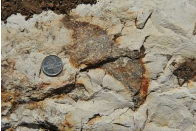
Figure 37. Wholesale quartz-albite replacement (white) of rhyolite porphyry (grey) illustrating resorption of original igneous porphyritic texture.
