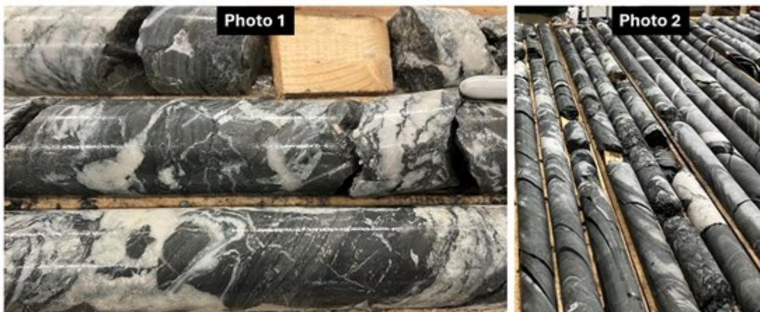
Photo 1 (Left): Example of multiphase vein development within deformed sediments. NQ sized core from
