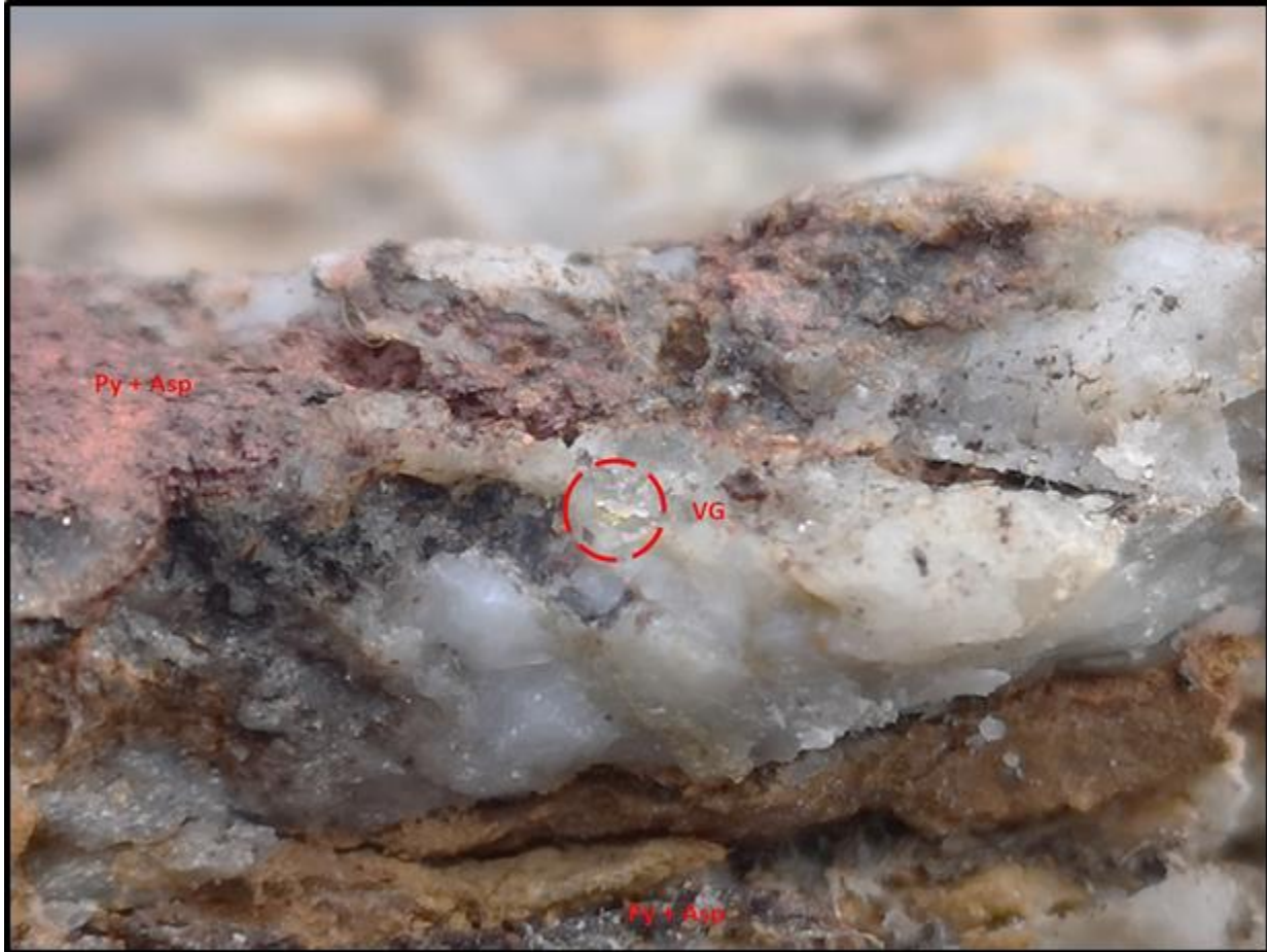
Figure 2: Example of fine-grained visible gold (VG) from the Quinlan Veins. Visible gold grains are <1 to 2 millimetres in diameter. Pyrite (Py) and arsenopyrite (ASP) are observed along the quartz vein boundary with the host rock and as minor veinlets within the quartz.
