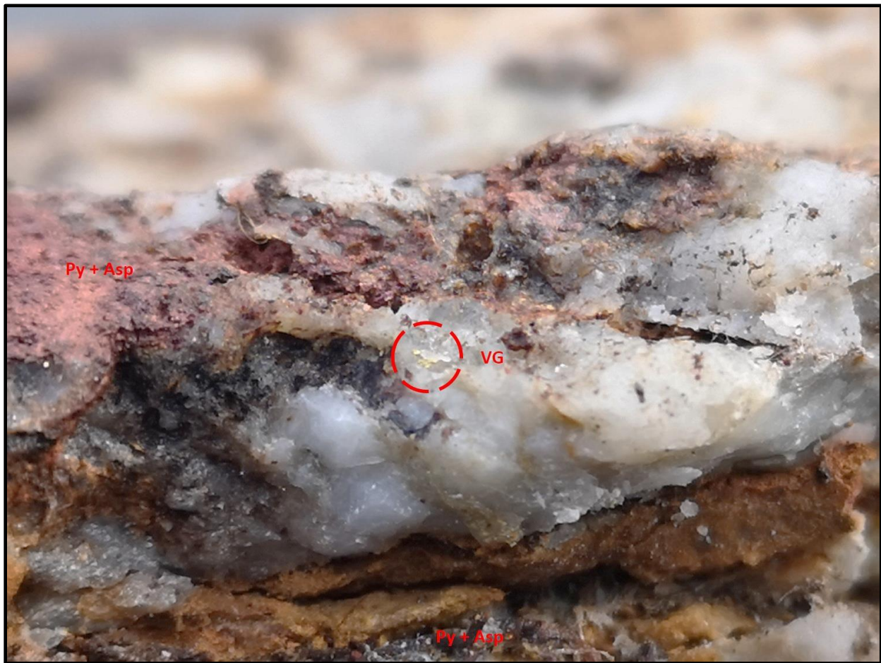
Figure 3: Example of fine-grained visible gold (VG) from the Quinlan Veins. Visible gold grains are <1 to 2 millimetres in diameter. Pyrite (Py) and arsenopyrite (ASP) are observed along the quartz vein boundary with the host rock and as minor veinlets within the quartz.
