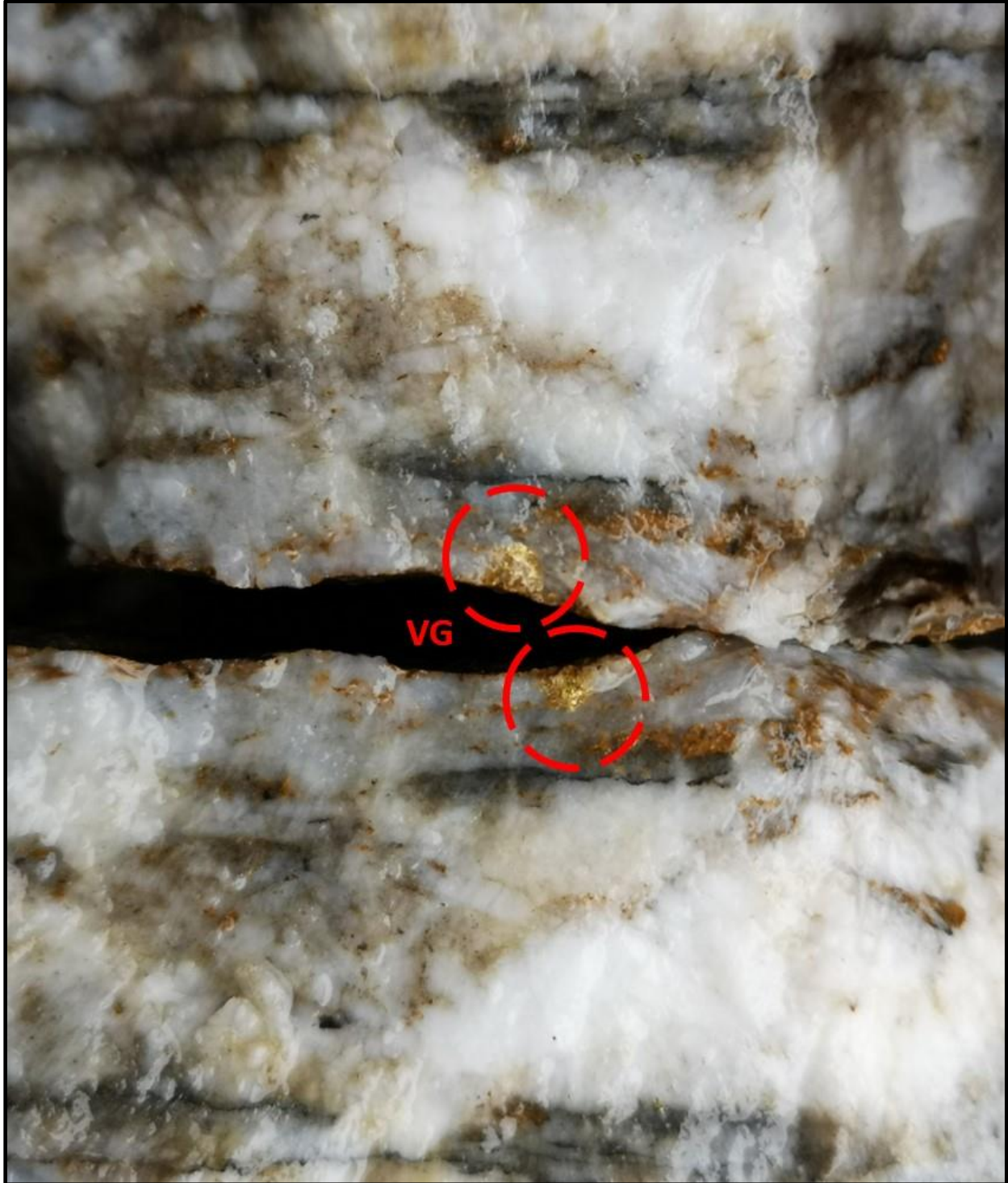
Figure 2: Medium grained visible gold (VG) from the Little Joanna Quartz Vein discovery in the Dog Bay Gold Project. Gold grains were observed between <1 millimetre and 3 millimetres in diameter. Black shale inclusions and sulphide stylolite veinlets are typical in the quartz veining.
