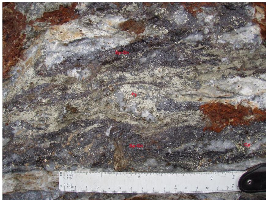
Figure 2: Massive sulfide containing sphalerite (Sp), galena (Gn), chalcopyrite (Cp), and pyrite (Py) from historical trenching at the Black Bart prospect.
