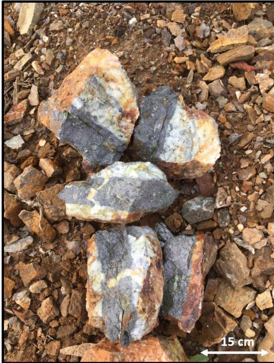
Figure 3: Arsenopyrite bearing quartz from the JP vein. Sample was assayed at Eastern Analytical using package ME-ICP41, aqua regia digestion followed by ICP-AES analysis; PGM-ICP24 and ran 7.71 g/t Au.
