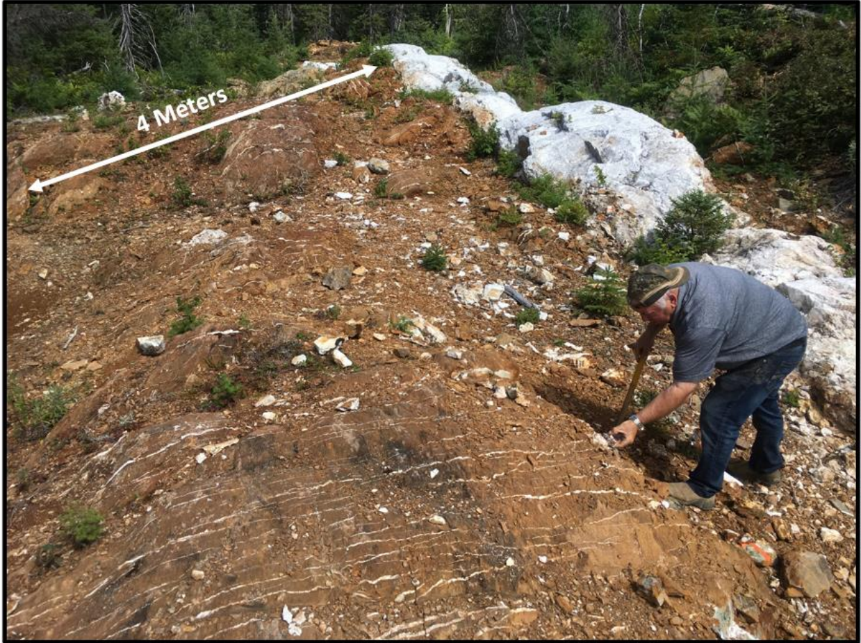
Figure 2: Silicified gabbro rock unit in contact with JP vein. Best Assay 14.42 g/t Au and was assayed at Eastern Analytical using analytical package ME-ICP41, aqua regia digestion followed by ICP-AES analysis: PGM-ICP24.
