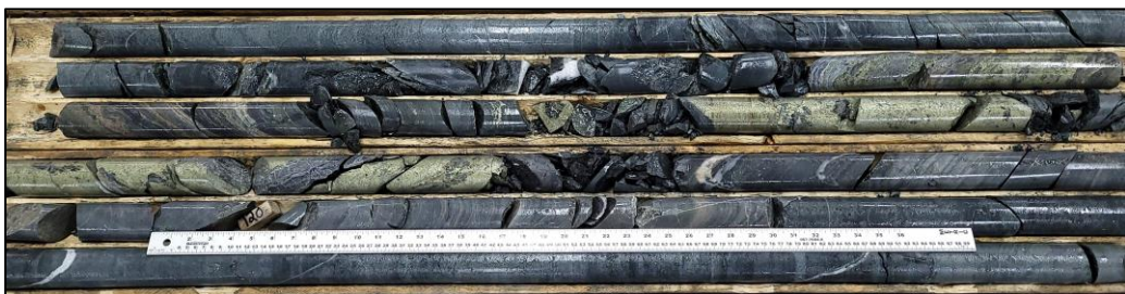
Photo 2. Zone 2 massive and stringer chalcopyrite between 116.55m and 119m in DDH CC03-23
