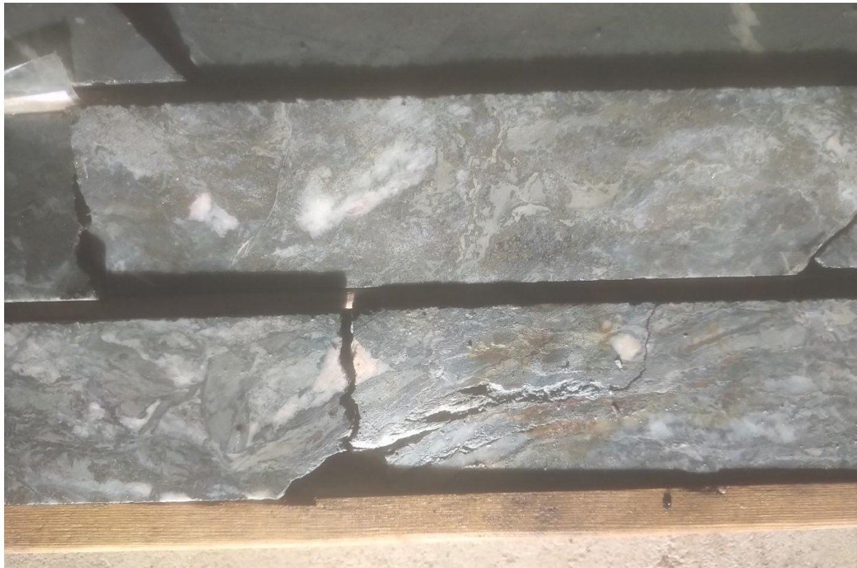
Figure 12-1: DDH BG11-47, 294.5 – 295m, chaotic silicified quartz fragmental Fe-Zn-Pb semi-massive sulphides (Sample 1058302).
