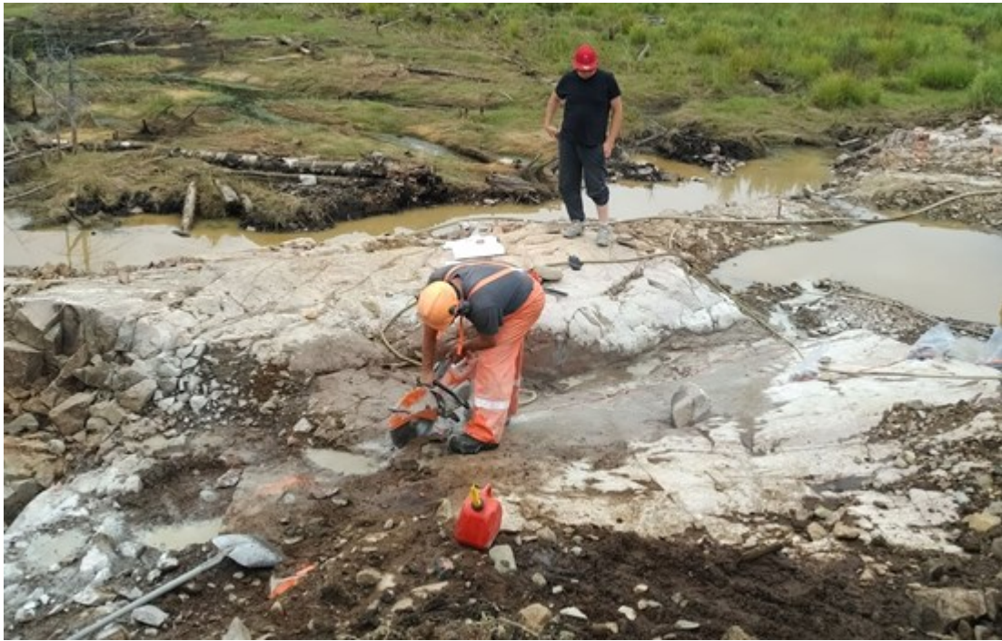
Photo 1. Channel Sampling of the Allied Syenite
