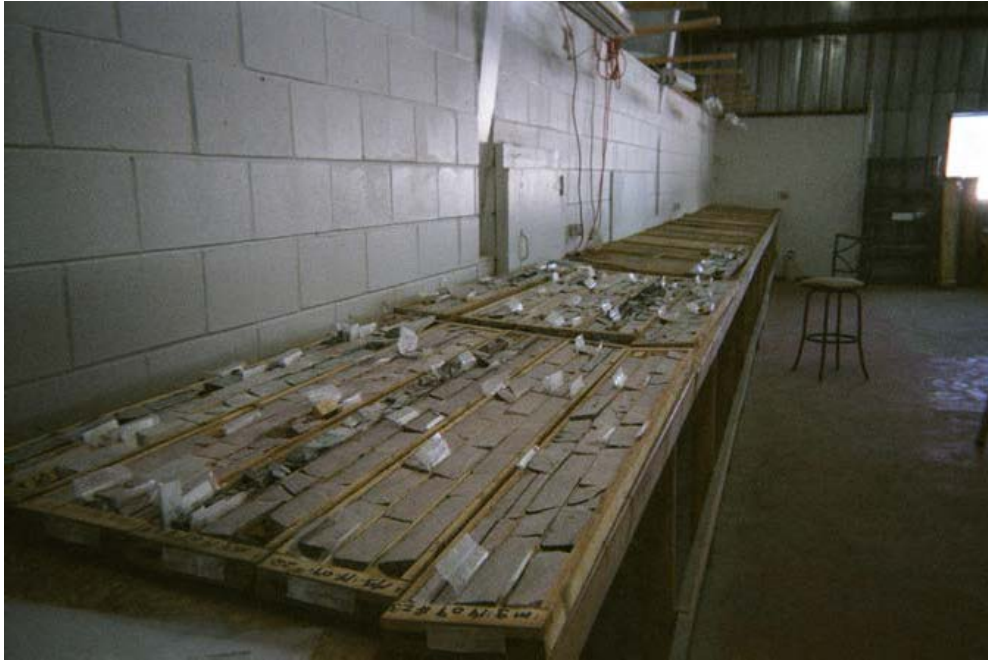
Figure 12-18 Drill core racks for logging and sampling inside storage warehouse.
