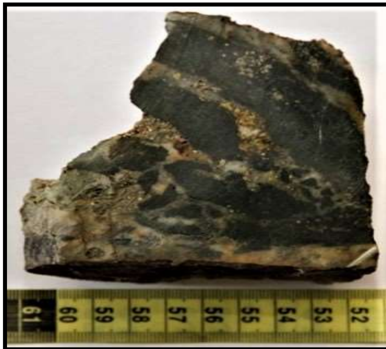
Figure 4: Surface exposure of quartz-calcite-sulphide breccia within chloritic shear at the Pinnacle Showing. Sample# 1964 containing 2.54% Cu, 7.78g/t Au, 12.3g/t Ag and 5.00ppm Mo.
