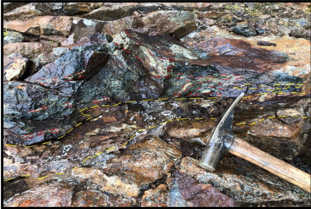
Figure 5: Surface exposure of mineralized chloritic shear zone at the Pinnacle showing. Dashed yellow lines delineate a southeast striking moderate southwest dipping oxidized quartz-carbonate vein. Dashed red lines highlight pyrite-arsenopyrite mineralization.
