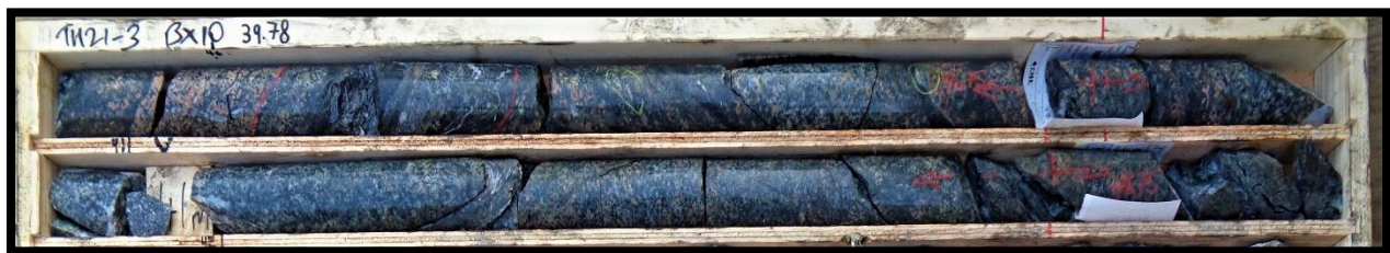
Figure 3: Semi-massive magnetite vein infilling chloritic shear and crosscut by quartz-sulphide veins and fractures. TH21-3 from 39.78 to 41.75m.
