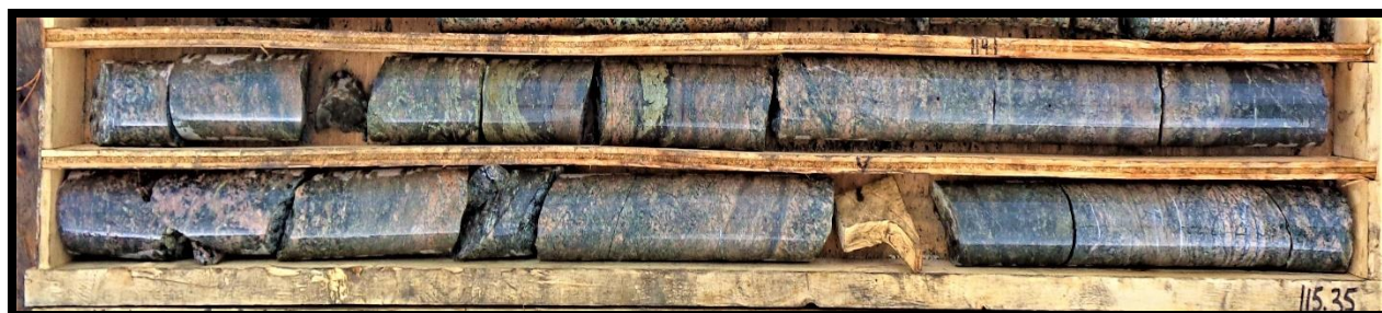
Figure 1: Isolated pyrite+chalcopyrite veins replacing magnetite with associated pervasive k-spar alteration proximal to chlorite shear within TH21-12. Sample# 42261 from 113.35m to 114.35m containing 0.75% Cu, 0.23ppm Au, 1.87ppm Ag and 63.00ppm Mo over 1.00 meter.
