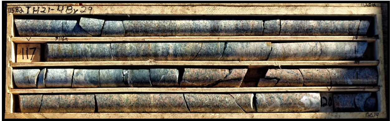
Figure 2: Low grade mineralization intersection from 115.82m to 120.14m within TH21-4. Mineralization occurs within patchy-pervasive albite and silica alteration proximal to chloritic shear on diorite-(quartz) monzodiorite contact.
