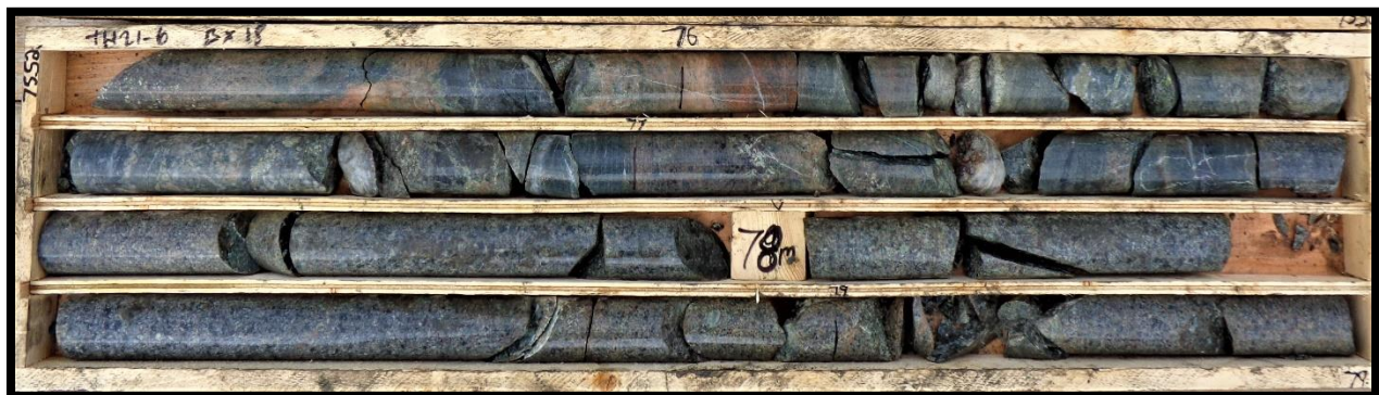
Figure 4: Hairline fractures, veins and coarse blebby pyrite and chalcopyrite within silica+calcite healed and brecciated shear structure within TH21-6. Sample #43035 from 75.77m to 77.00m containing 0.68% Cu, 0.06ppm Au, 2.62ppm Ag and 65.7ppm Mo or 0.78% CuEq over 1.23 meters.
