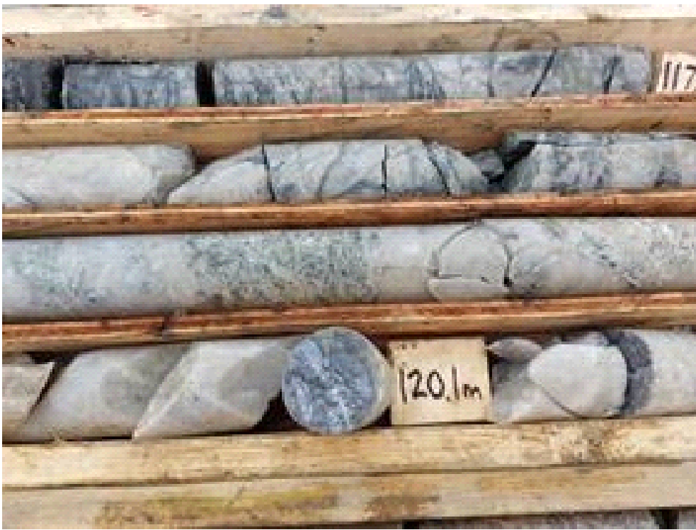
Figure 1: Representative photo of molybdenum mineralization identified near the end of drill hole NL-22-74
