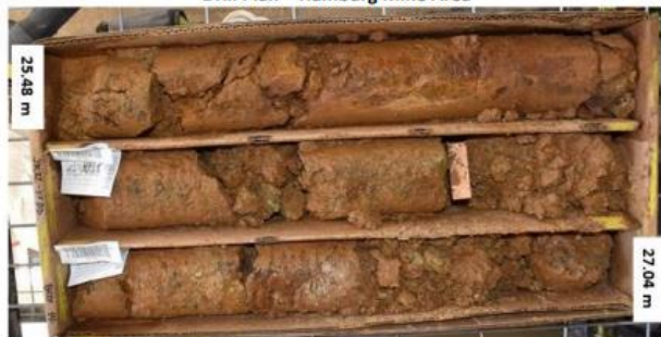
Gossanous CRD 24.57 m to 26.12 m, over 1.55 m, 9.42 g/t Au, 73.6 g/t Ag, 2.27% Pb & 2.27% Zn
