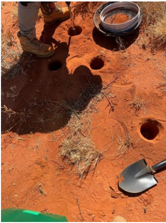
FIGURE 1: PHOTOS FROM SITE VISIT TO ARTIC FOX & ISBJORN PROJECTS - Note: Auger holes and sampling on the auger traverse at Isbjorn Project (Source: Megawatt geology team) (CNW Group/MegaWatt Lithium and Battery Metals Corp.)
