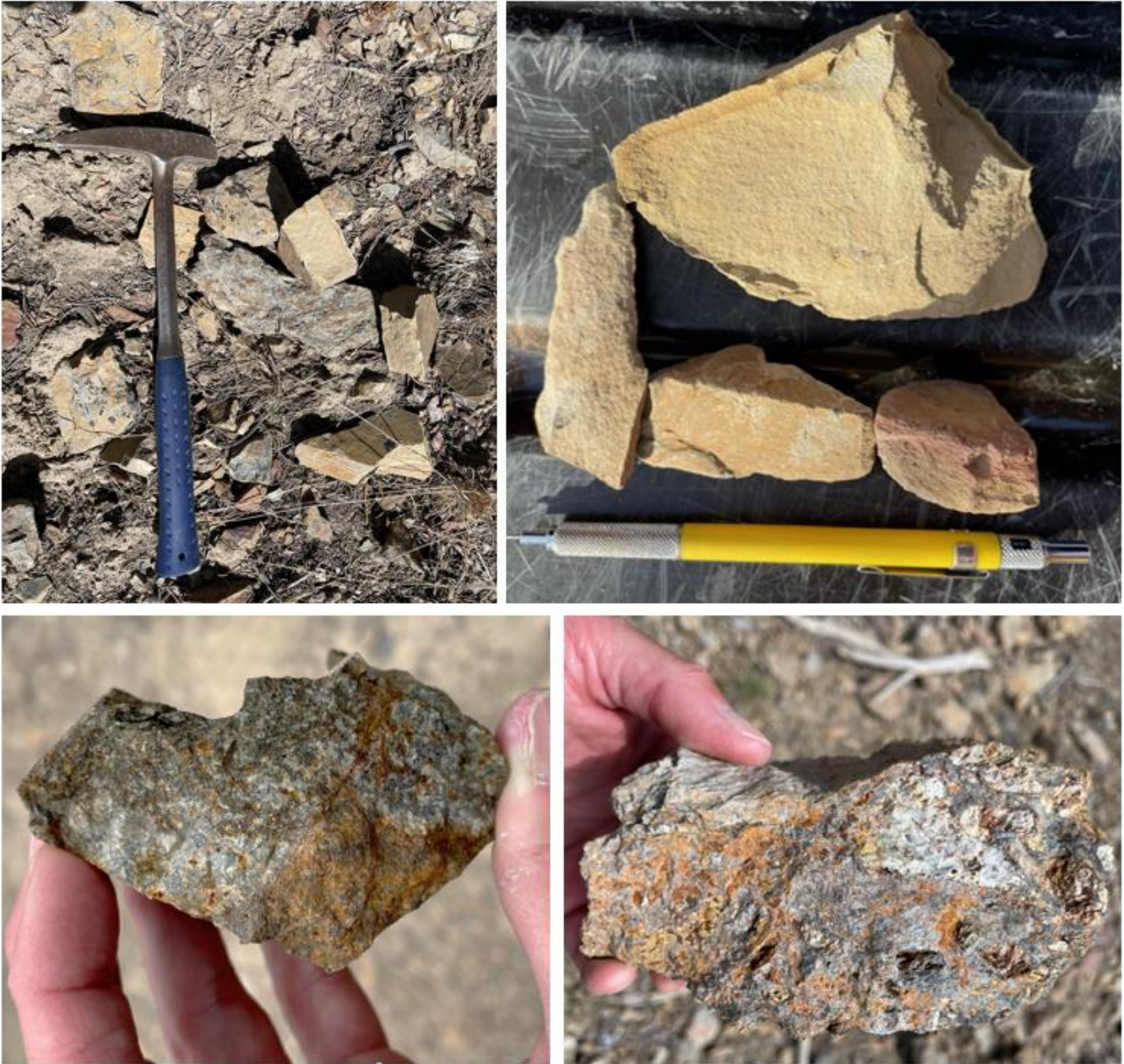
Figure 2 (Top): “Punky” decalcified and oxidized Wenban Formation silty limestone
