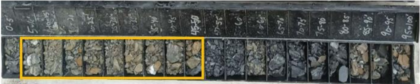
Figure 5: Oxidation Observed in Hole T2202
