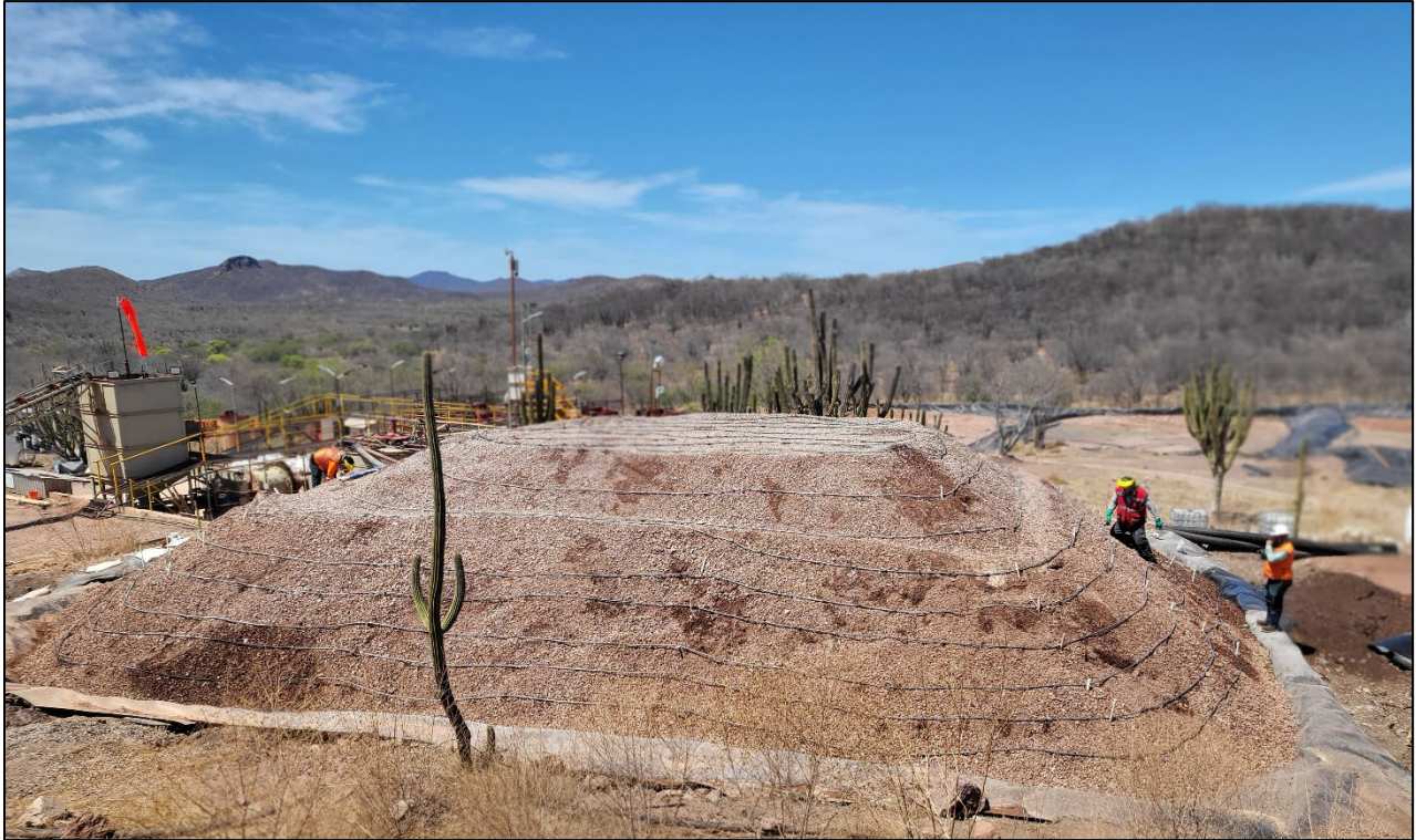
Plate 1. A. Bulk Sample heap leach pile. B. Testing solution during leaching. C. Initial loading of carbon in leaching tanks.
