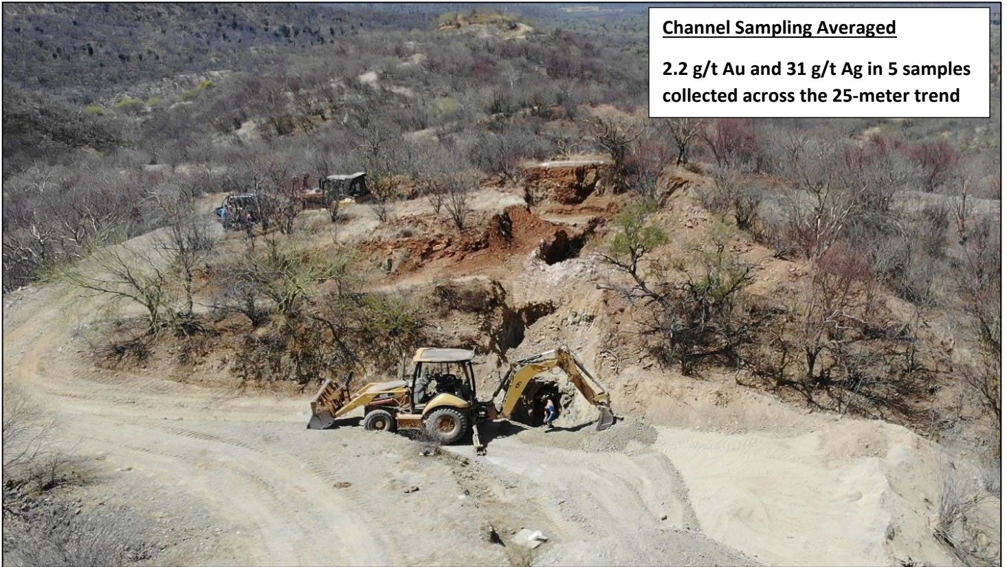
Photos 1 & 2. Above, Trenching for Bulk Sample at 4-T, channel sampling averaged 2.2 g/t Au and 31 g/t Ag over the 25-meter trend. Below, a stockpile of bulk sample material – Main Zone.
