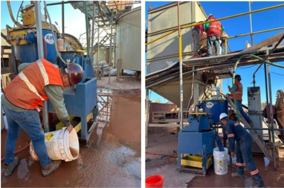
Photos 3 & 4 Above. Top left, gravity concentrator added to circuit for testing. Top right quartz vein rock sample collected from old working exposed during trenching.
