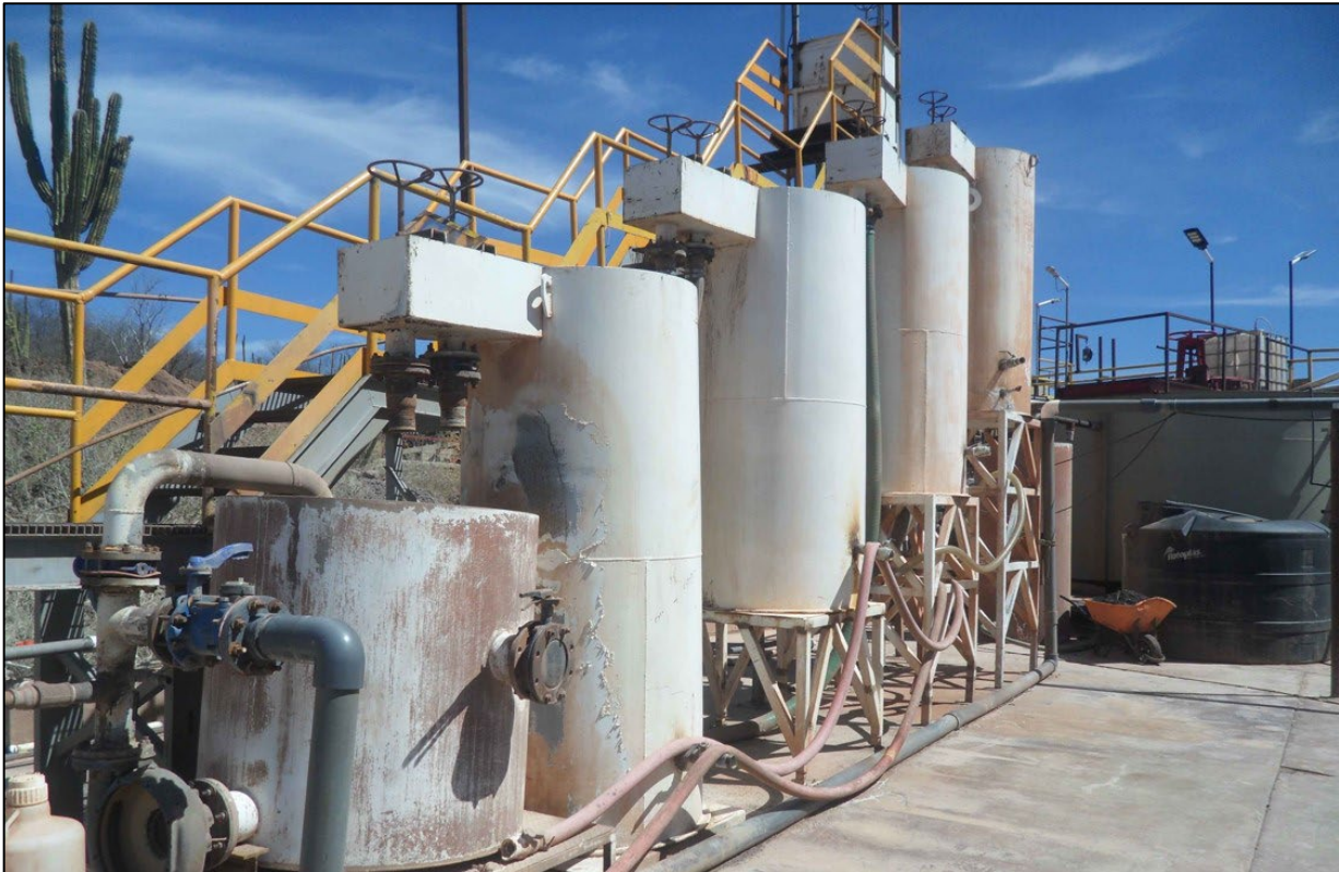
Photos 1 & 2. Above, Ground conditioning for heap leach pad. Below, Absorption Tanks for treating solution.
