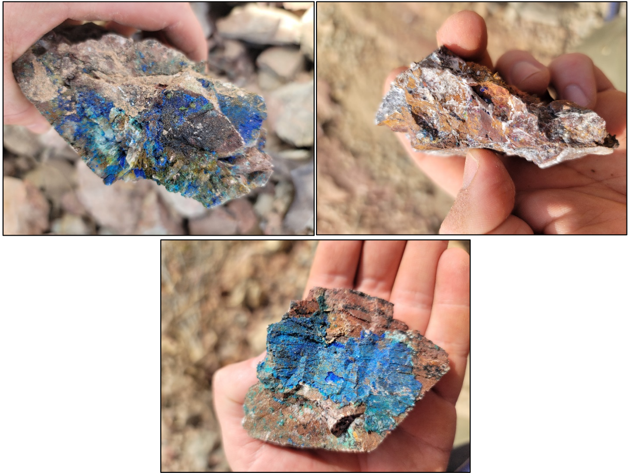
Plate 1: Photos of oxide mineralization at North Hill Prospect with secondary copper (malachite and azurite). Past surface sampling returned ranges of 0.35 g/t to 3.3 g/t Au, 13 to 178 g/t Ag and 0.09% to 1.1% Cu.
