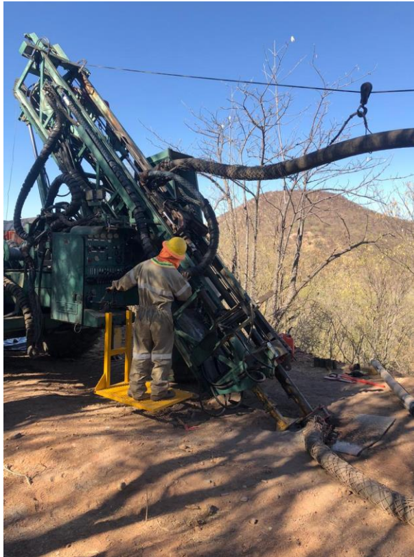
Photo 1. RC Drill Rig operating at the Pilar Gold-Silver Project.
