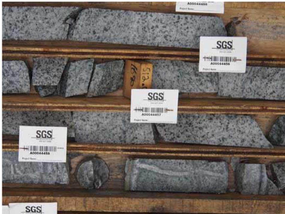
Figure 23: Stockwork Mineralization at the End of Drill Hole MRC-006
