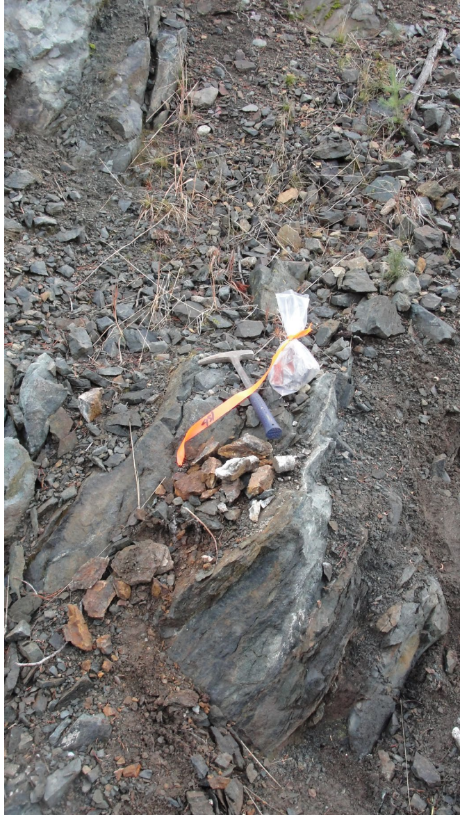
Photo 2. Sample site 451, Upper Road Area. This sample (0451 in tables 7 & 8) returned 841 ppb Au and >100 ppm Ag from a quartz vein cutting foliated ultramafic rocks of the Tulameen Complex. Photo taken by C. Lynes, November 2016.
