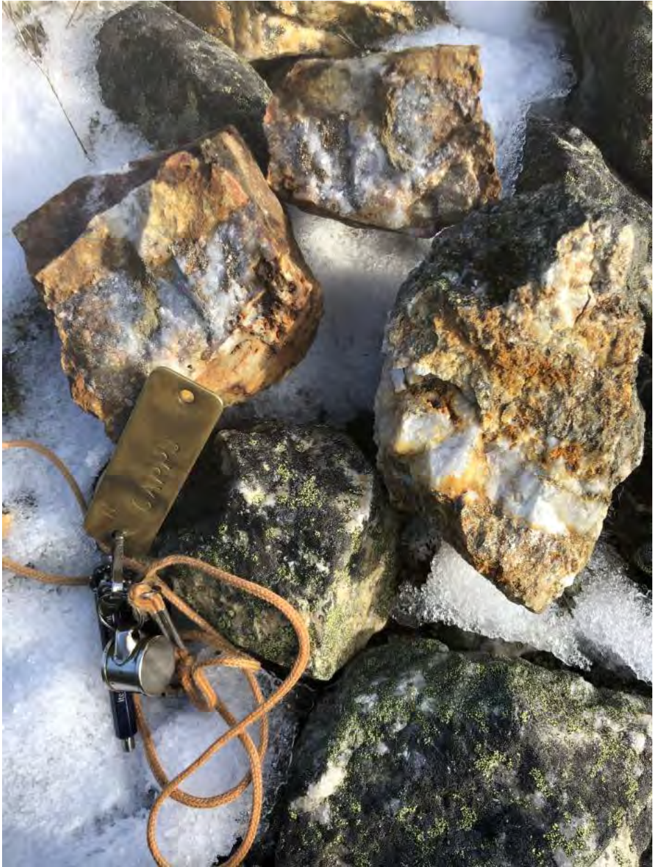
Figure 14: Broken boulder of vein material showing oxidized sulfides and veining from historic placering along streams form deposits several meters deep at the Mary K prospect(see Tables 5 and 7 for gravity concentration)
