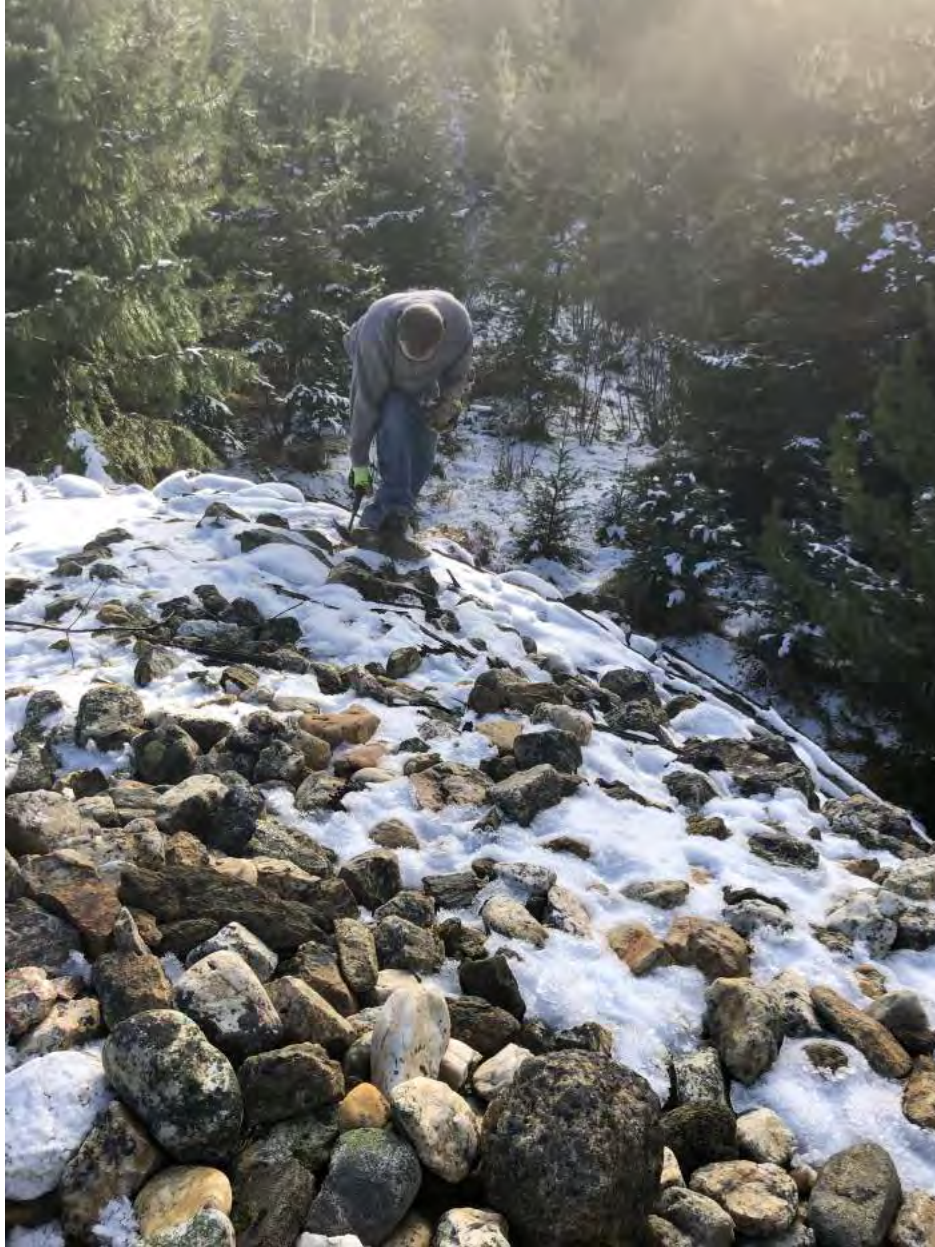
Figure 13: Extensive boulder tailings from historic placering along streams form deposits several meters deep at the Mary K prospect (see Tables 5 and 7 for gravity concentration)
