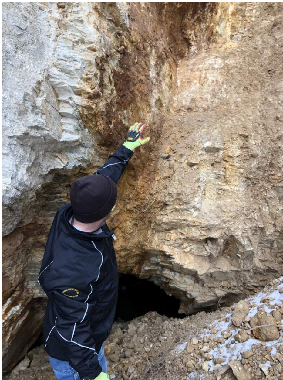
Figure 10: Photo taken looking northeast along the strike of the Mary K vein and shear zone at the Level 1 portal, of the historic Mary K mine. MJ Mining geologist Brooks Hintze is indicating the northeast-striking and steeply northwest-dipping shear zone along the vein. Note the moderate northeast dips of gneissic foliation to the left of Brooks Hintze and in the hanging wall of the shear and Mary K vein. The gneissic foliation is nearly perpendicular to the trend of the vein.
