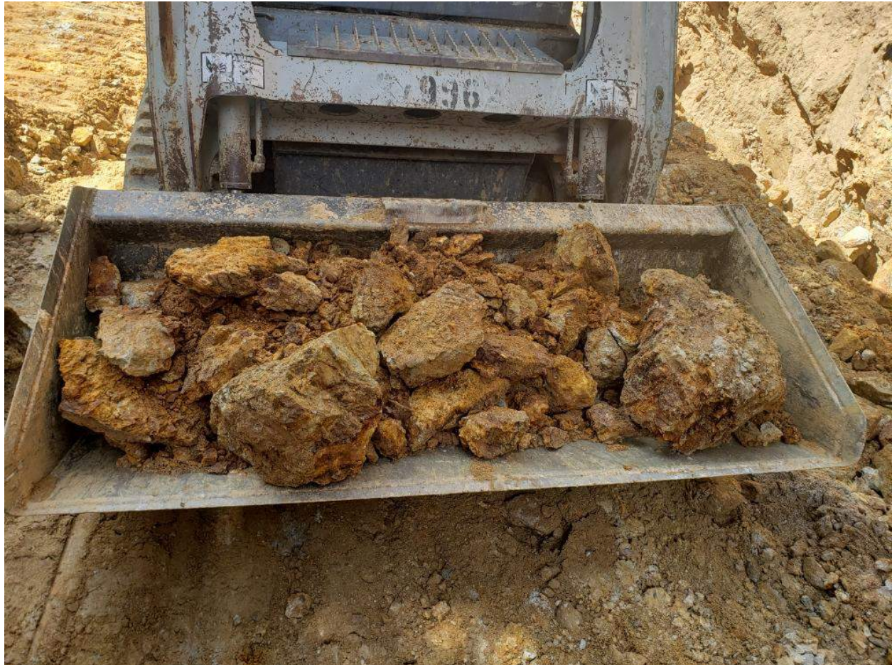
Figure 16: Bulk sample of Mary K vein being transported to the gravity circuit (see Tables 3 through 14)
