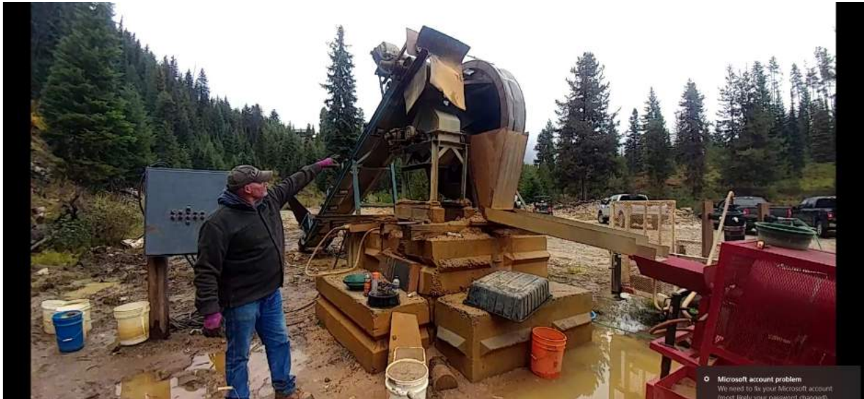
Figure 17: The Mary K bulk samples are crushed and then processed through a Reverse Helix gravity circuit to produce the concentrates(see Tables 3 through 14)
