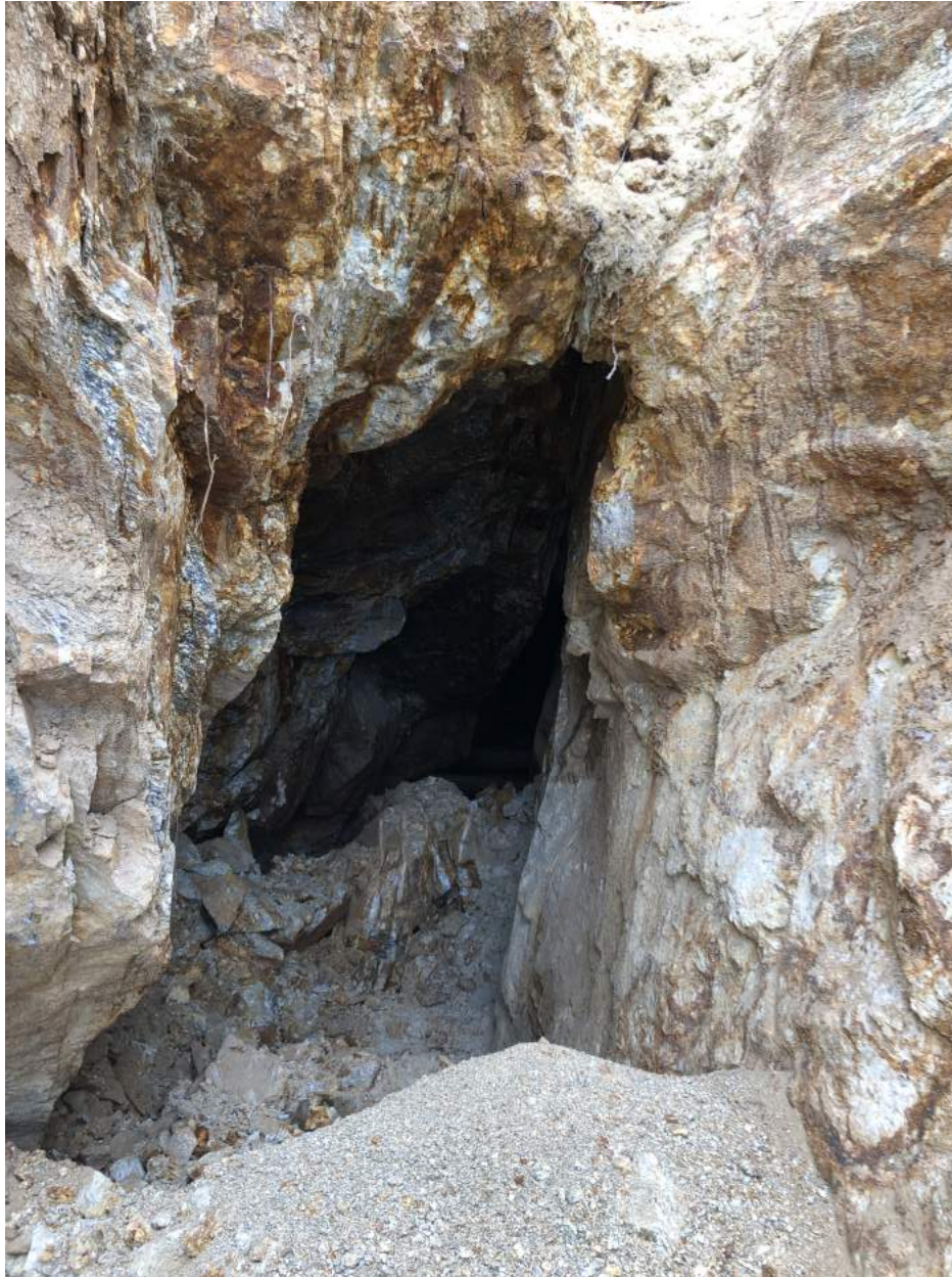
Figure 8: Portal to the lowermost main tunnel (Level 4), at the historic Mary K mine. View to the northeast along strike of vein and shear zone. Vein and shear zone dip steeply to the northwest. Gneissic foliation dips moderately to the northeast.
