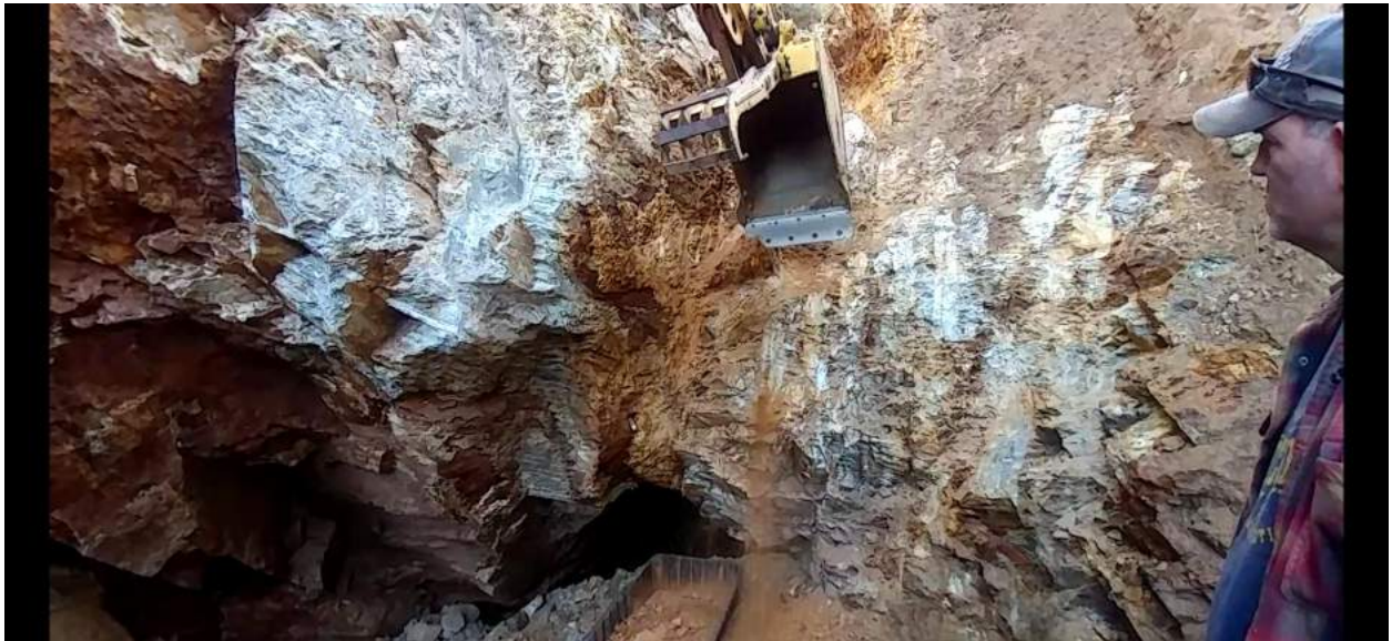
Figure 15: Surface bulk sampling along the Mary K vein at the Level 1 portal (see Tables 3 through 12)
