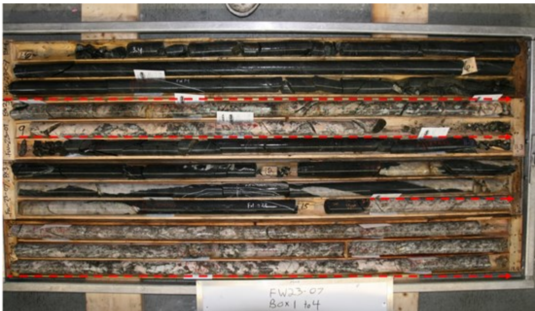
Figure 2. Core showing high-grade (1.5% Li 2 O) spodumene mineralization in Hole FW23-07 (Far West North "FVN" Pegmatite)
