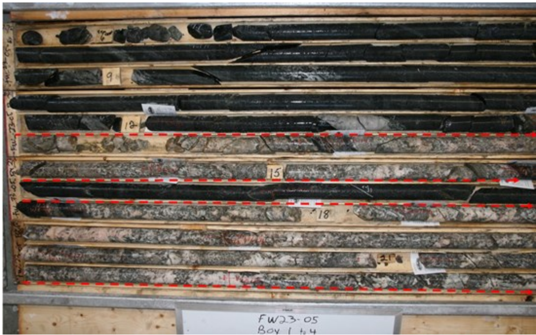
Figure 1. Borehole FW23-05 Core Samples showing high-grade (>1.3% Li 2 O) spodumene mineralization (Far West South "FWS" Pegmatite)
