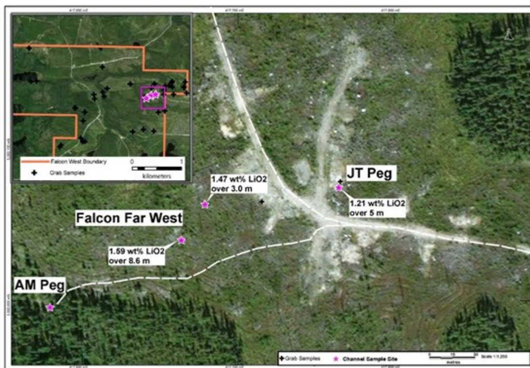
Figure 1. Satellite photo map showing the location of the channel sampling sites on the Falcon West Lithium property. The significant Li 2 O % intervals are reported on the map.
