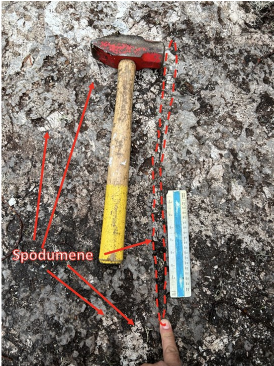
Figure 2. Large (up to 50cm) Spodumene (primary Lithium mineral) crystals in the newly discovered AM spodumene pegmatite showing which comprise approximately 50% of the rock mass in the outcrop.
