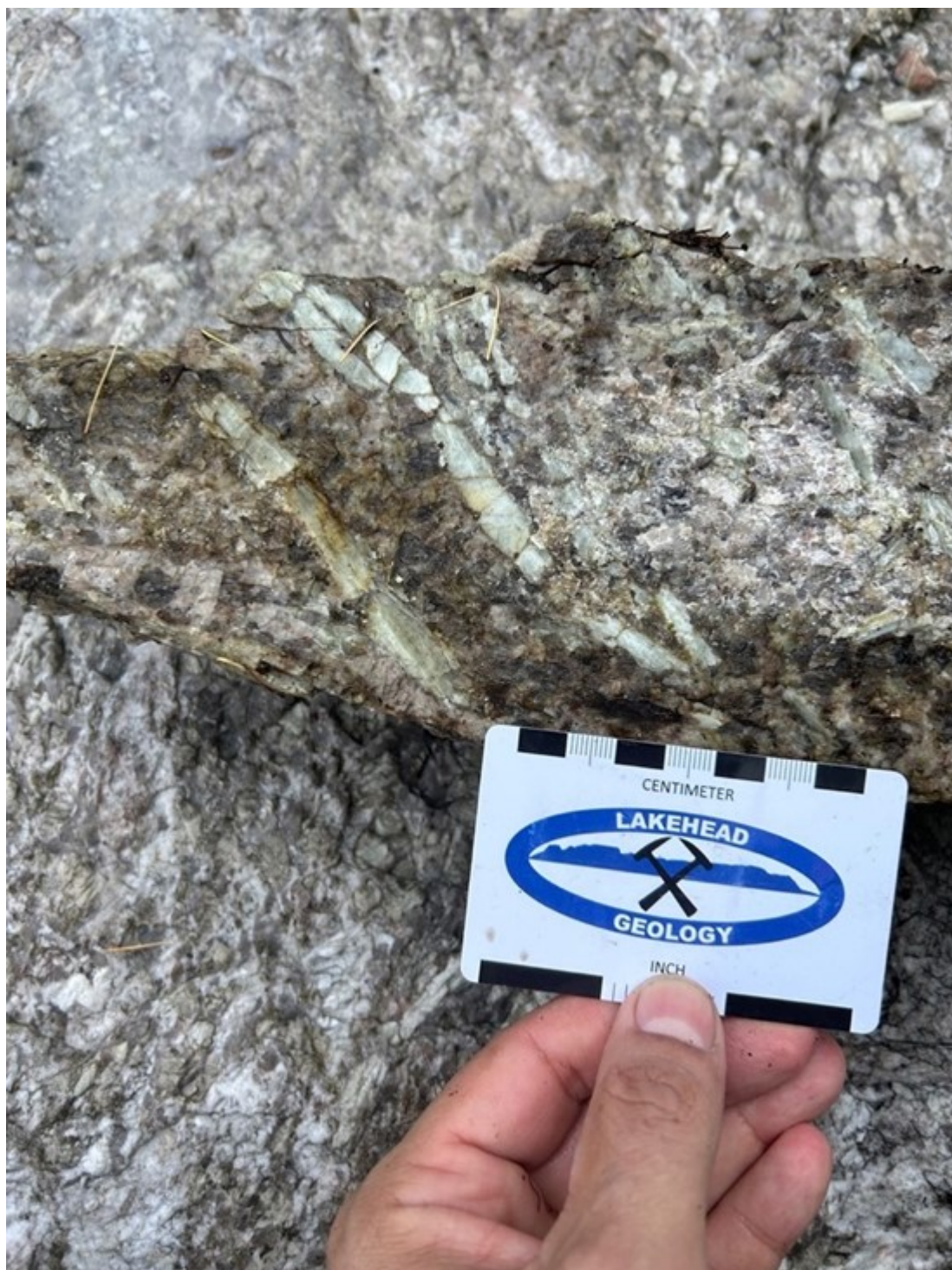
Figure 2. Pegmatite outcrop on Volta's Falcon West Lithium Property containing large Spodumene crystals (primary hard rock Lithium mineral)
