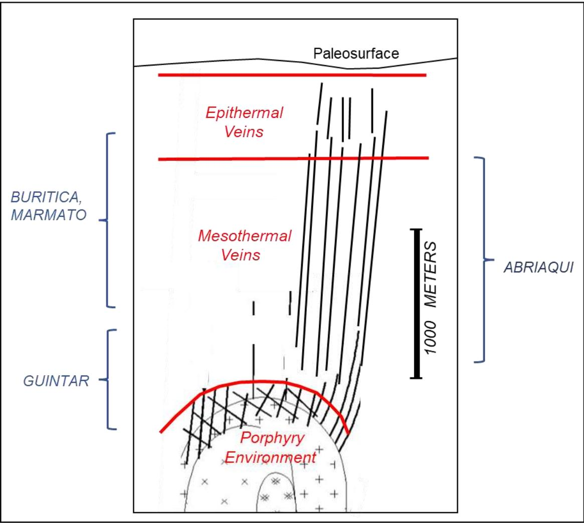
**Figure 1.** Idealized schematic of porphyry gold-copper system with associated veins (modified after Corbett, Sillitoe). The estimated vertical extent of exploration is shown for the four deposits included in Table 1.
