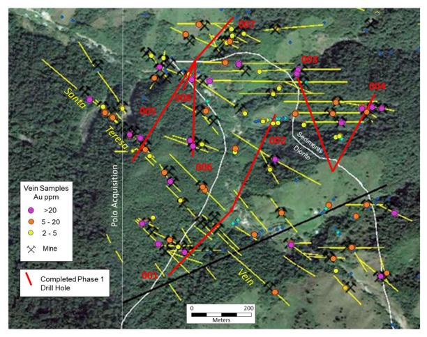
Figure 1. Phase 1 Drill Holes Completed through January, 2021
