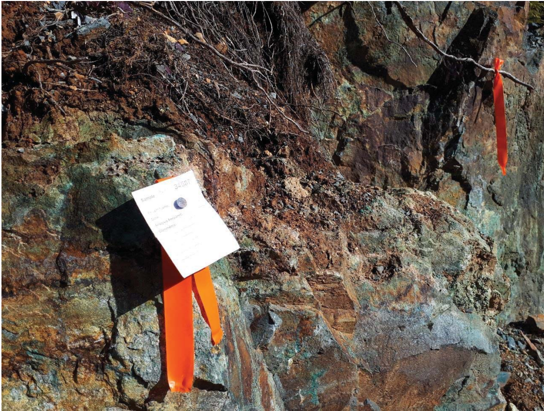
Photo 3. Green malachite staining in outcrop at sample site 34507, Eclair showing. This sample site returned 5.27% Cu and 24 ppm Ag. Photo taken by the Author, April 25, 2018.
