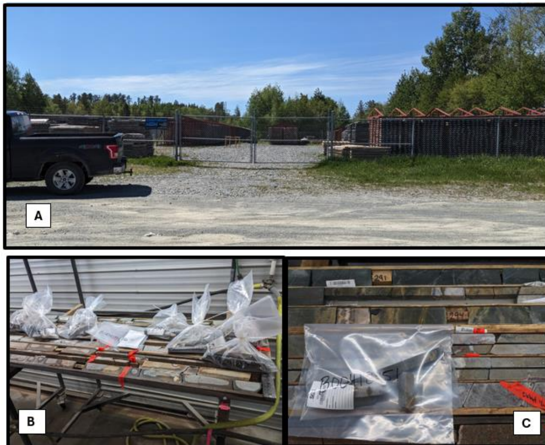
Figure 12.1 – A) Fenced and locked enclosure where the Swanson project core is stored. B) Bagged sample at the Explo-Logik core shack. C) Quarter core sample taken from hole SW-22-014.
