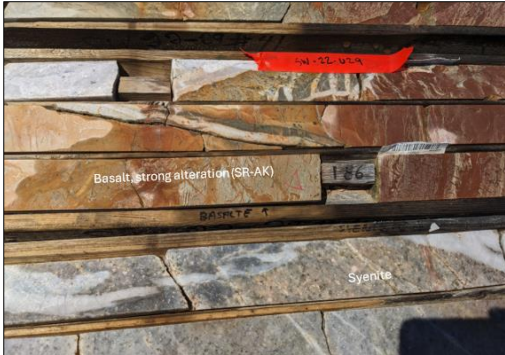
Boundary between two lithological units, strongly altered and mineralized basalt and a porphyritic syenite.
