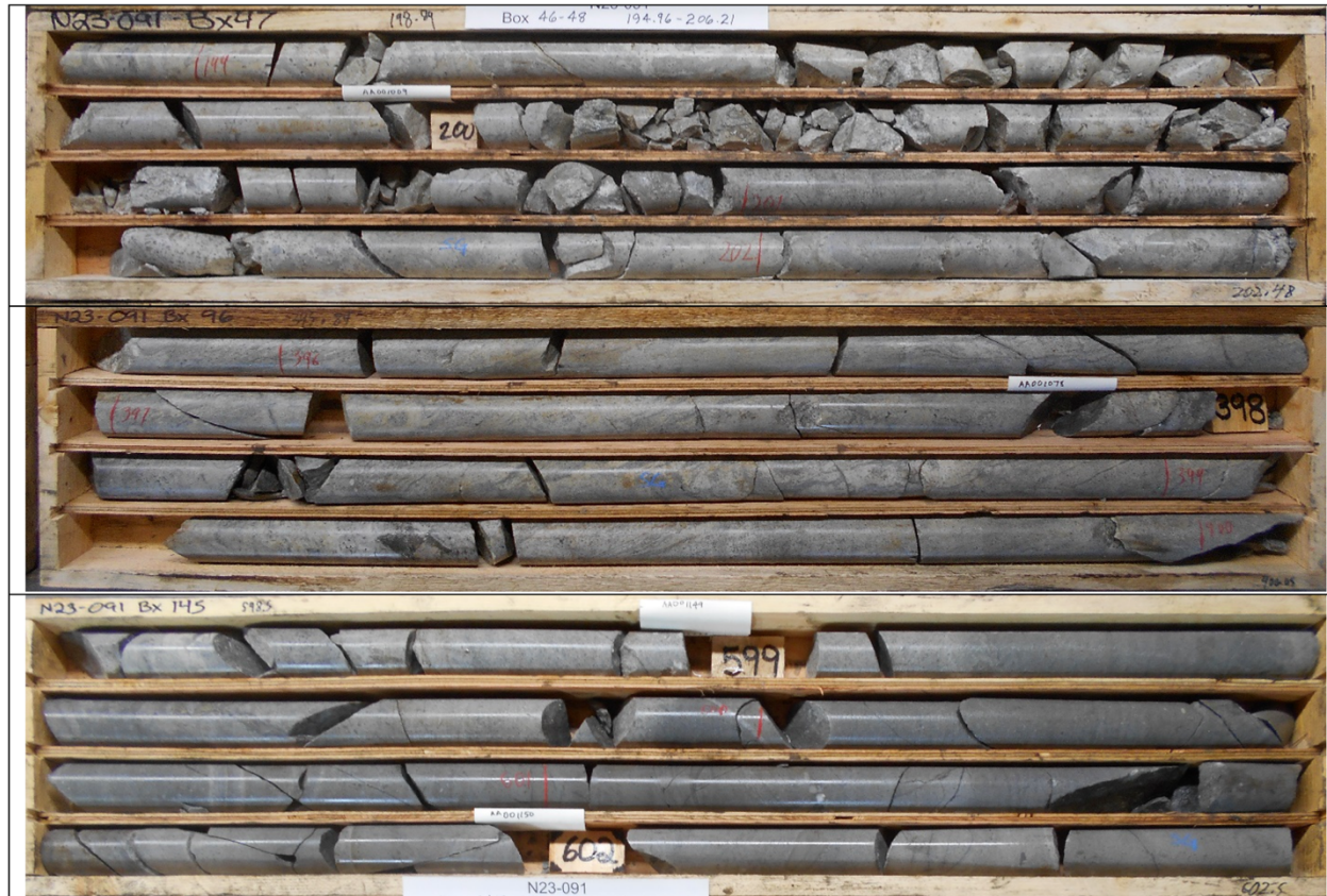
Figure 3: Quartz sericite altered felsic volcanics with disseminated and vein controlled pyrite – marcasite sulphides. These are select small sections of the core within the felsic volcanic units that were intercepted being shown here for demonstrative purposes.
