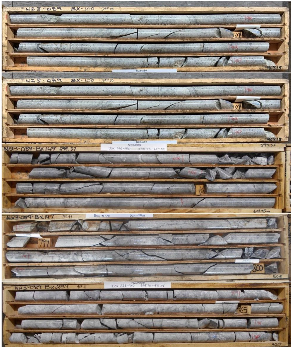
Figure 2: Quartz sericite altered felsic volcanics with disseminated and vein controlled pyrite – marcasite sulphides.
