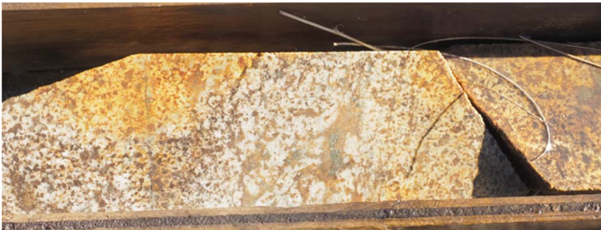
Figure 12-7 – ARGILLIC ALTERATION IN MONZONITE (HOLE 9004)
