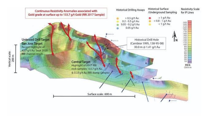
Figure 1: 3D view of northeast trending IP resistivity zones across the Cerro Magallanes dome. 100m line spacing with 50m spacing dipole spacing shows several shallow anomalies. The red lines are showing the primary mineralized trends correlated with the resistive anomalies in the IP sections.
