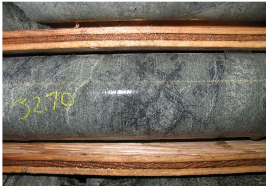
Plate 7-4: Dark colouration due to carbonaceous contamination along crackle breccia fractures in diorite. Carbonaceous material likely originates from graphitic argillite/mudstone unit 25 centimetres below. Drill Hole RR09-107, at 32.70 metres.
