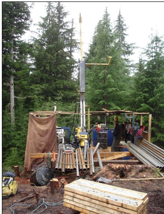
Plate 10-1: Blackhawk Drilling JT2000 diamond drill, collar for RR09-105, October 2009.
