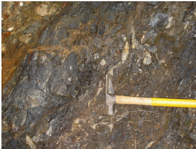
Plate 7-2: Photo of 4 metre chip sample locality (0.24 g/t Au, 14.7 g/t Ag, 498 ppm As, 656 ppm Cu, 571 ppm Pb and 1720 ppm Zn) on south bank of the Iskut River, just east of Baseline 3000E of the 150 Grid. Rock is graphitic argillite with disseminated pyrite, chalcopyrite and traces of sphalerite and galena and lies in the structural footwall stratigraphy to the main Black Dog horizon.
