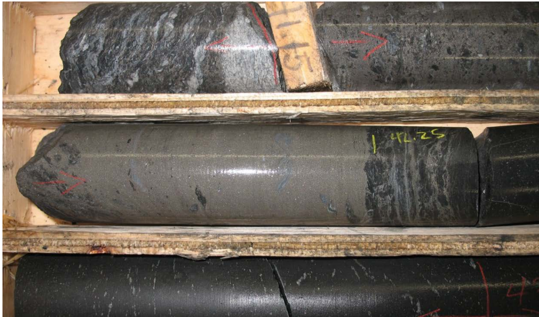
Plate 7-8: Photo shows variable textures of mudstone-minor siltstone-quartz clast breccia with massive pyrrhotite-minor chalcopyrite-sphalerite matrix and distinct bands (beds?). Section occurs at around 41 m in RR09-107, immediately above the laminated massive sulphide in Plate 7-7.
