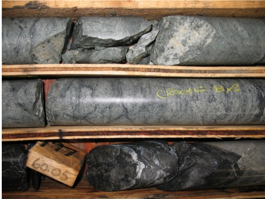
Plate 7-4: Dark colouration due to carbonaceous contamination along crackle breccia fractures in diorite. Carbonaceous material likely originates from graphitic argillite/mudstone unit 25 centimetres below. Drill Hole RR09-107, at 32.70 metres.
