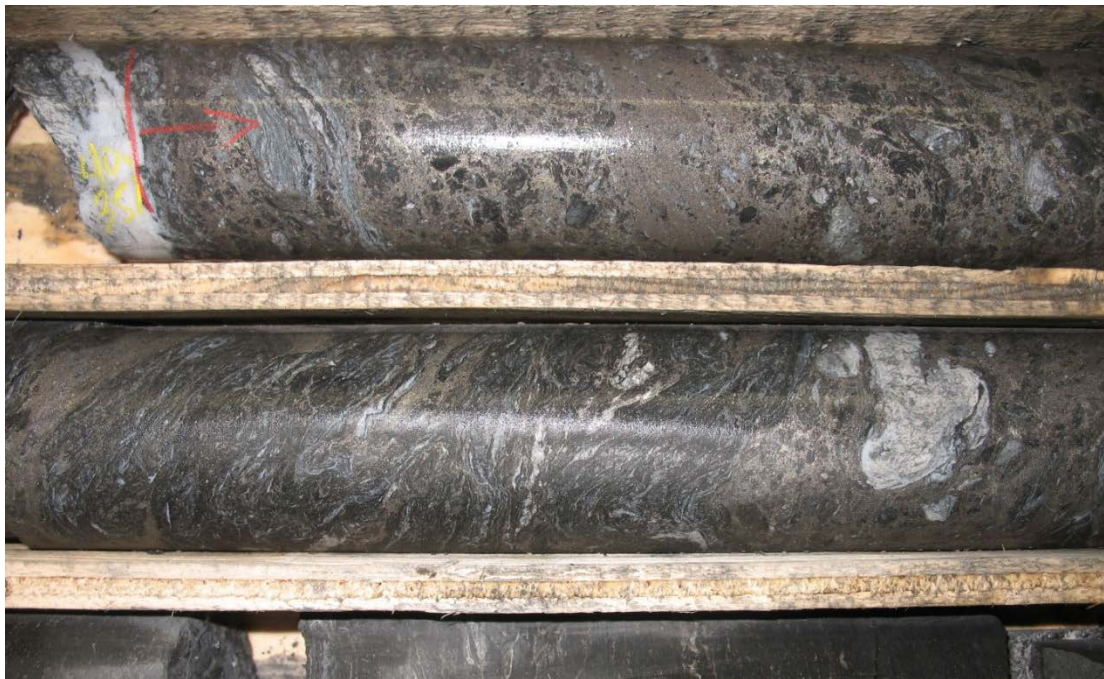
Plate 7-8: Photo shows variable textures of mudstone-minor siltstone-quartz clast breccia with massive pyrrhotite-minor chalcopyrite-sphalerite matrix and distinct bands (beds?). Section occurs at around 41 m in RR09-107, immediately above the laminated massive sulphide in Plate 7-7.
