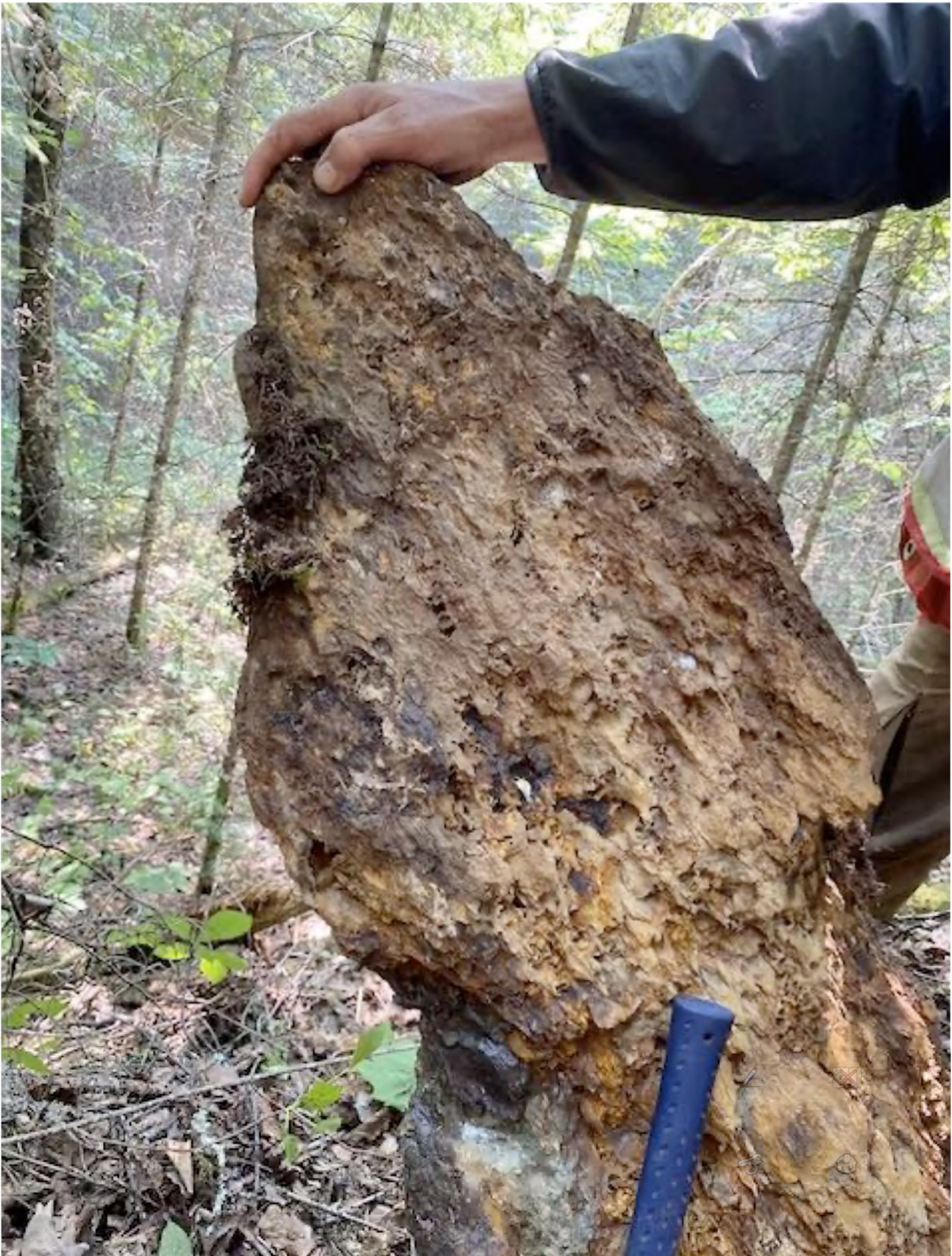
Photo 3: Rusty gossan boulder with up to 40% interstitial pyrite in brecciated silicified intermediate volcanics. Peninsula Bay Area believed to be near the Mongus Lake Au, Cu discretionary occurrence.
