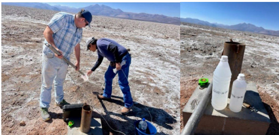
Figure 11.4 Bailing sample from Well INCA-21-05R (22 March 2022) (MACL, 2022)
