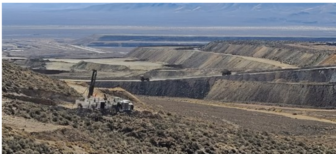
Figure 1: Drill Rig (foreground) with Nevada Gold Mines' SXEW Copper Leach Pad, Mine Dump and Tailings Pond in Background. (Source: Golden Independence)
