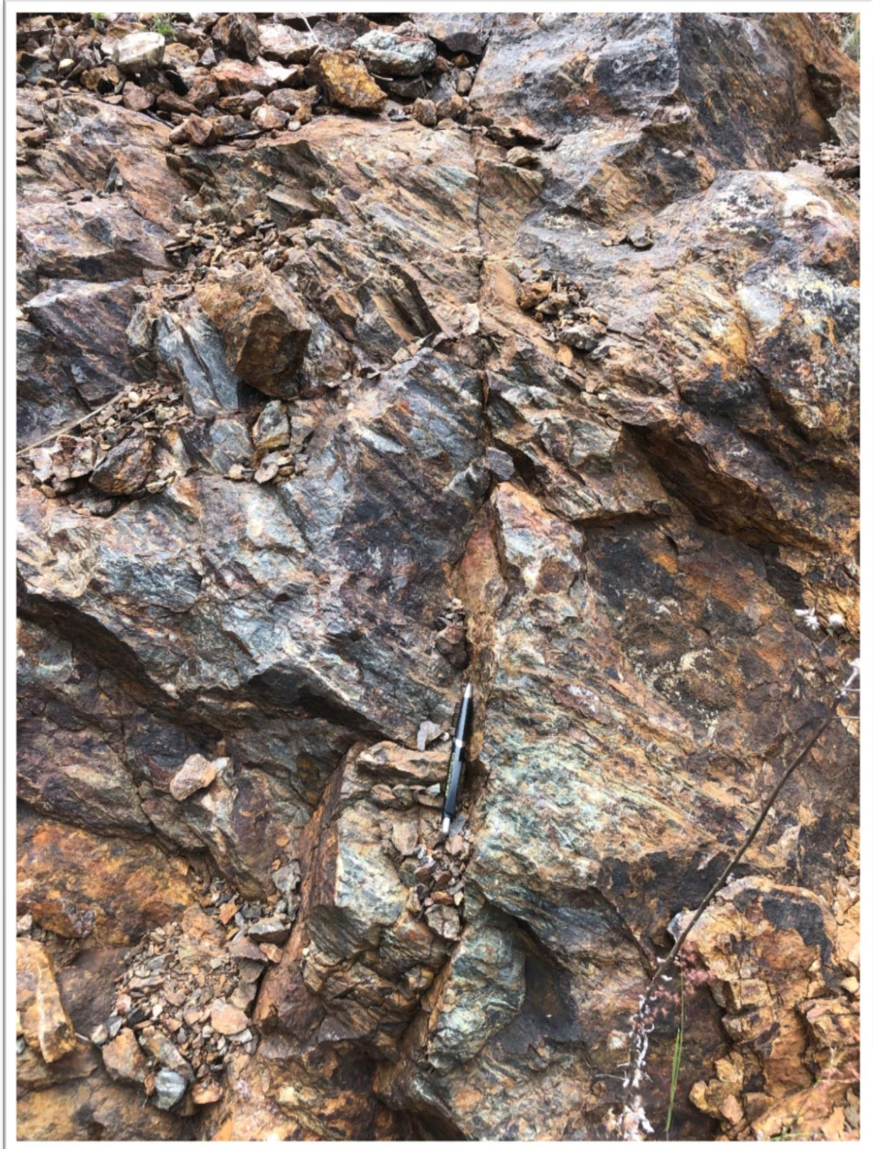
Figure 7.10: Chlorite Schist at Wanga - NE trending Jointing shows FeOx on Surface (source Geosure November 2019).
