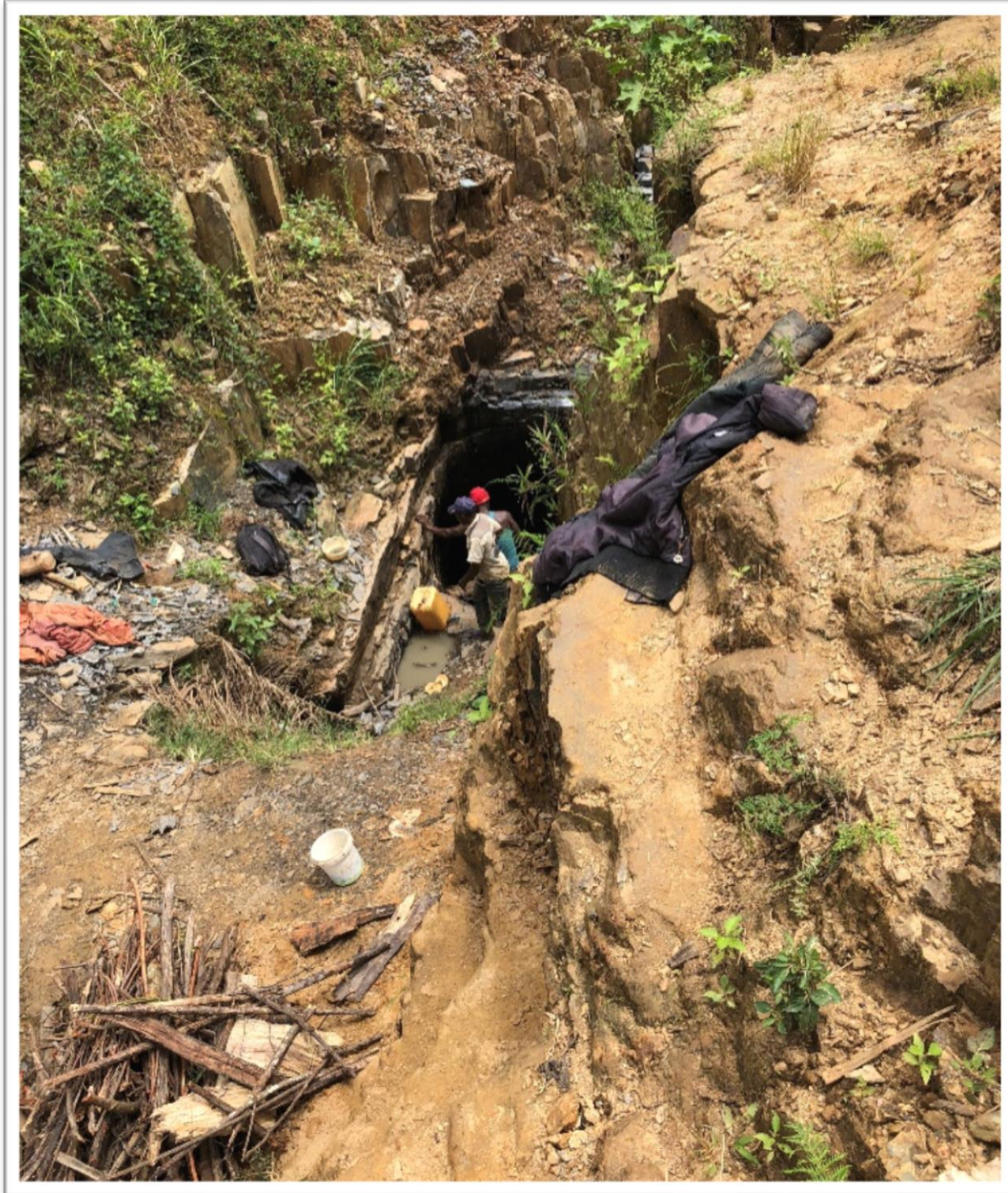
Figure 7.9: Artisanal Miners Exploiting NE Trending Quartz Veins at Wanga (Mondial) (source Geosure November 2019).
